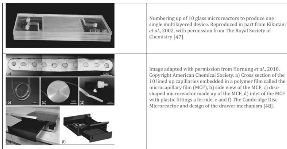
Figure 1.7 Examples of multiple microreactors used in parallel for higher throughput and yield of products [47,48]. Source : Figures reprinted with permission, copyright (2010), American Chemical Society.
