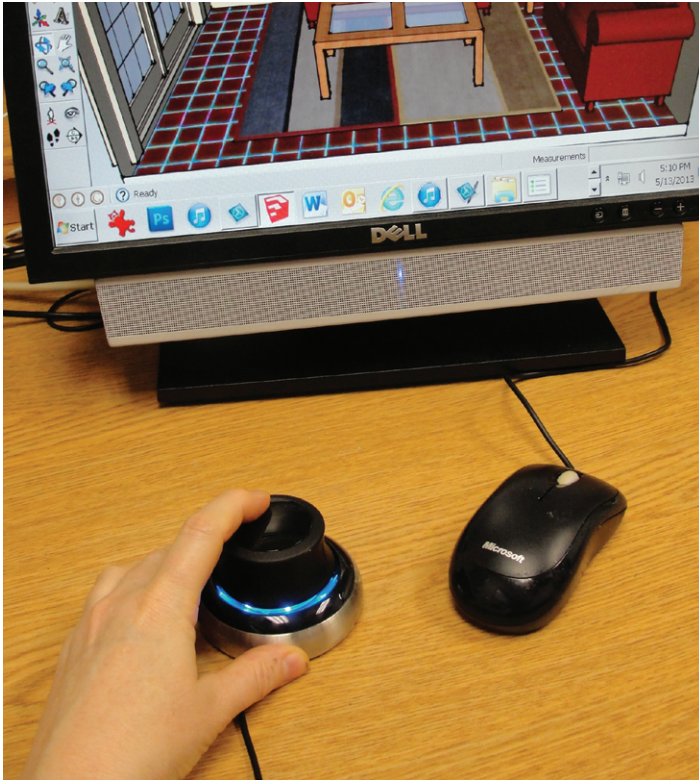
Figure 2-2: The Logitech Space Navigator 3D mouse moves through the model more efficiently than the traditional mouse, and can be used alongside it.
