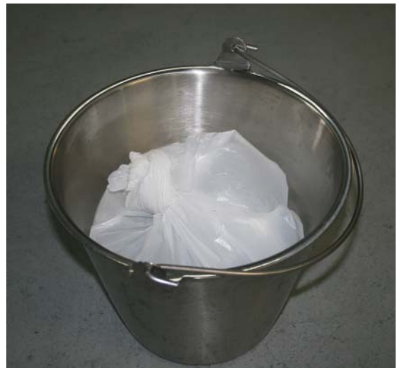
Figure 3.9 Bucket with liner closed to prevent dirt from contaminating water or to prevent water spillage when walking quickly with the bucket.
