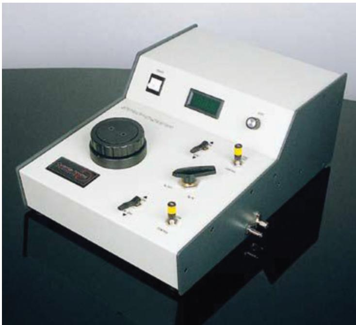
Figure 1.2. A Quantachrome® manual pycnometer.
