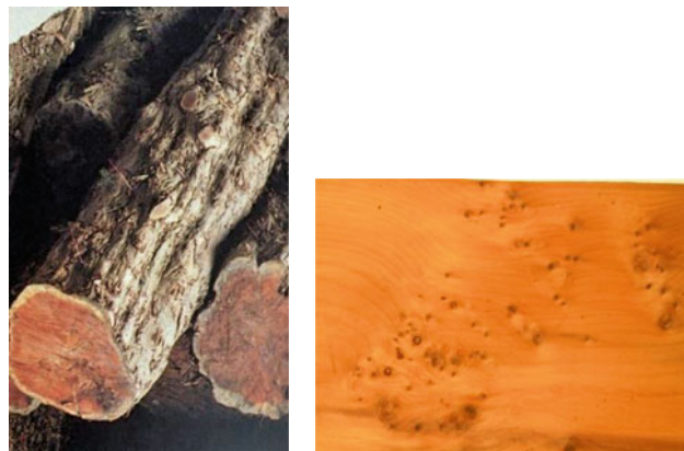
Fig. 2.3 A yew ( Taxus ) stem with many small branches (twigs, suckers) can be used to make valuable burl veneer. In this case, the cluster of knots is seen as a desirable wood characteristic
