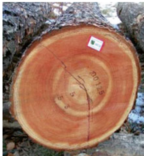
Fig. 3.17 Larch ( Larix ) missing pith leading to "moon rings" (Germany)
