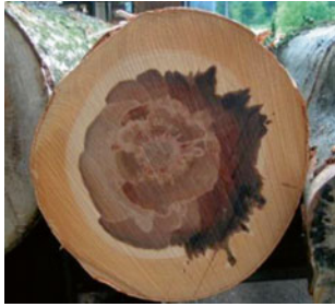
Fig. 3.15 Beech ( Fagus sylvatica ) with facultative red heartwood, visible as cloud heartwood, and pathological rot (black colored)
