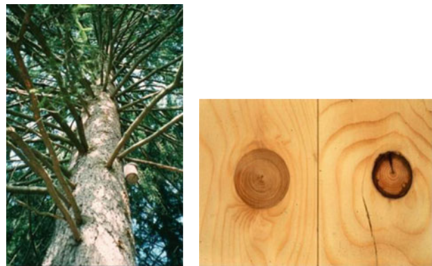
Fig. 2.2 Not all branches are equal: This limby spruce will (only) provide lumber full of ingrown and black knots. A branch – at least one with the dead black knot – is seen as a wood defect
