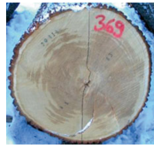
Fig. 3.16 Oak ( Quercus robur ) with incomplete pith formation
