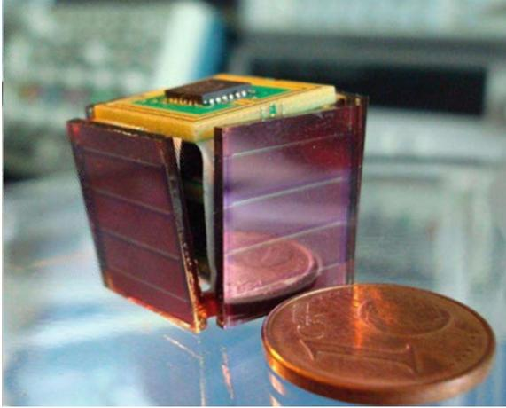
**Fig. 1.1** Illustration of a sensor cube application integrating photovoltaic harvesters as packaging [34] (reproduced with kind permission of Valer Pop)
