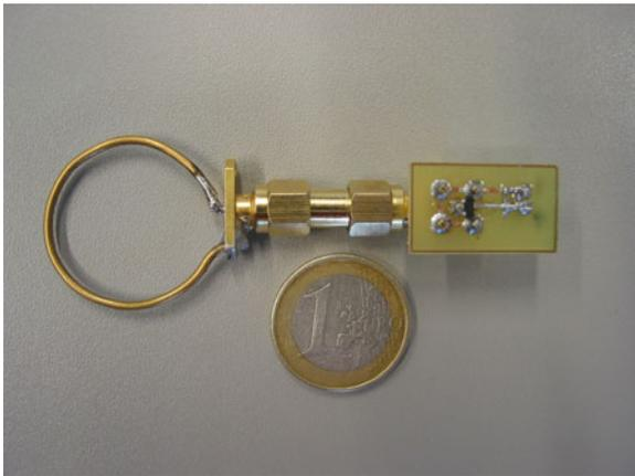
**Fig. 1.3** RF harvesting system with a small loop antenna (reproduced with kind permission of Tolgay Ungan)
