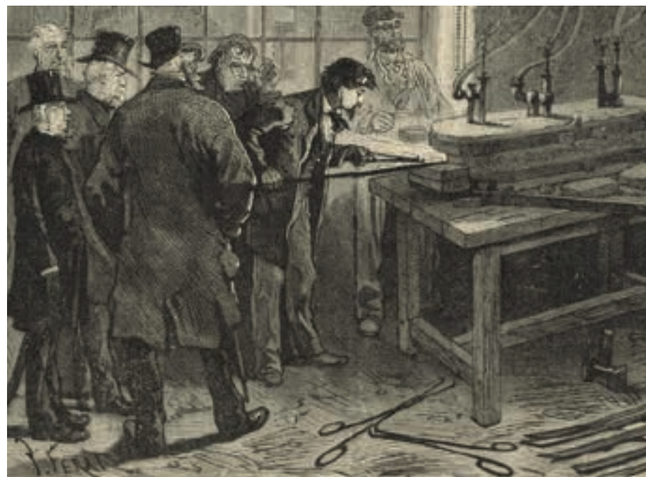
Casting the international meter bars in Paris. Wood engraving from 1874.
