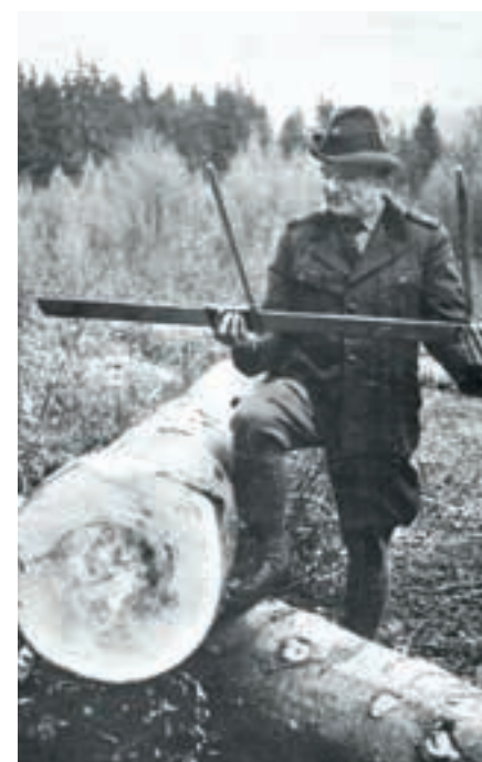
A Mahr tree caliper in use. The photo dates from a later period, but the principle behind the instrument has not changed since it was first developed.
