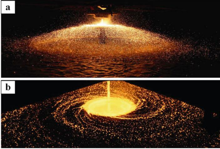
**Fig. 2.6** (a) 30 t/h centrifugal atomization of steel with water quenching and (b) top view on large cup with metal flow (from [25] with permission)
