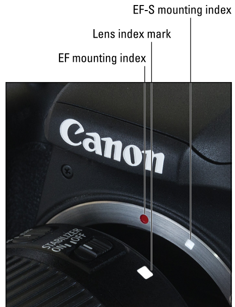
FIGURE 1-1: Align the mounting index on the lens with the one on the camera body.
