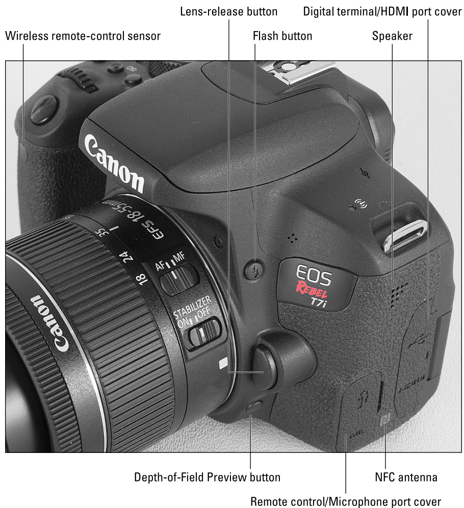
FIGURE 1-8: Other important controls reside on the front and left side of the camera.
