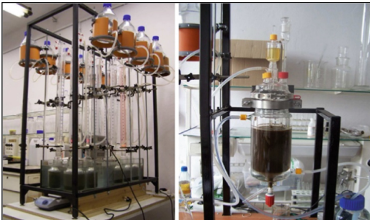
Fig. 1 Research stand for the study of biogas productivity of substrates according to DIN 38414 S.8 (left), inoculum station for quasi continuous fermentation work (right) Source own work
