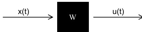
Fig. 15 The “black-box” approach. Here x(t) is an input signal, u(t) is an output signal, W is a hysteresis operator
