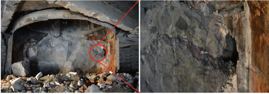
Fig. 6 Tapping channel of silicon through a more than 1 m wide slag layer
