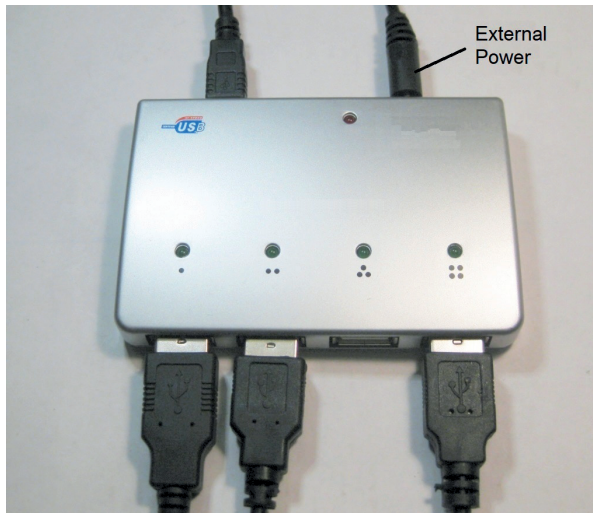
Figure 5.1: An active USB hub.
