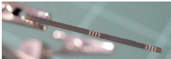
Figure 1.1.7: This PCB has a thickness of 1.6mm, and is made of fiberglass.
