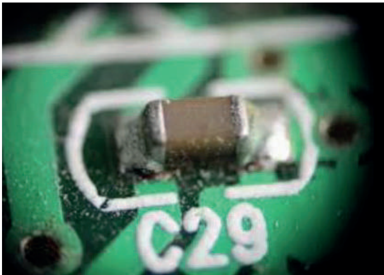
Figure 1.1.3: A surface-mounted component attached to a PCB.
