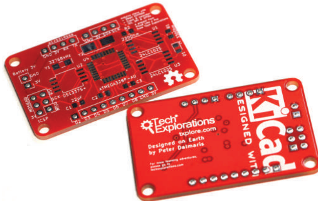
Figure 1.1.4: The white letters and lines is the silkscreen print on this PCB.
